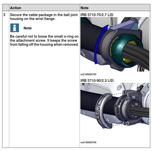
Fitting the cable package in upper arm tube
