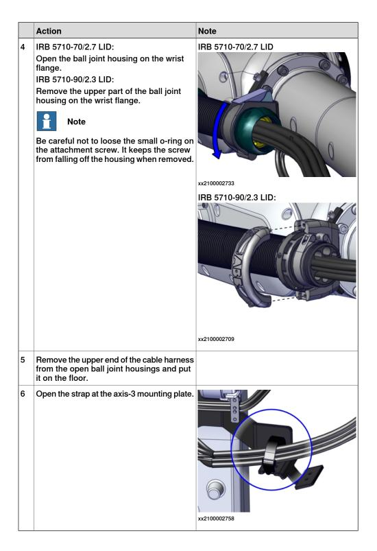
Removing the protection hose (protection type Foundry Plus)
