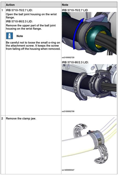
5.4.2 Replacing the protection hose for LeanID MH cable package *Continued*
