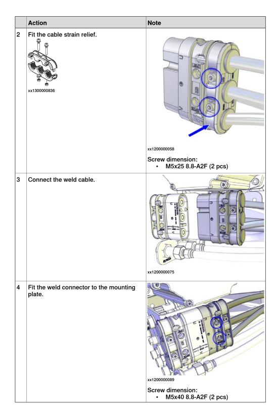
Connecting and securing the cable package to the upper arm
